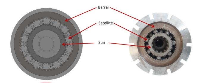
In this system, the SUN makes the rotation movement. The section defined as the BARREL is fixed and the screws, which are defined as STARS, rotate around the axis of its own as well as around the axis of the sun. Thus, the polymer materials, which are forced into the planetary extruders section and are in powder form, are brought to the melt form by mixing together with the shifting motion of the star and the sun and being subjected to more controlled shear stress.
